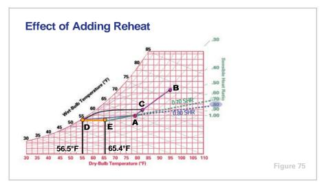
This supply air mixes with room air along the part-load 0.70 SHR line from **E** to **A**, arriving at the desired room conditions **A**. Now, if the room's latent heat gain were also changed, the resulting room conditions would not fall exactly on **A**, but on the appropriate SHR line that runs through **E**.
