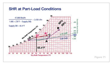
In response to the reduction in room sensible heat gain, the coil capacity is throttled, raising the supply air temperature from  $\mathbf{D}$  to  $\mathbf{D}'$  to balance the new room sensible heat gain. This new supply air temperature is dictated by the equation:
