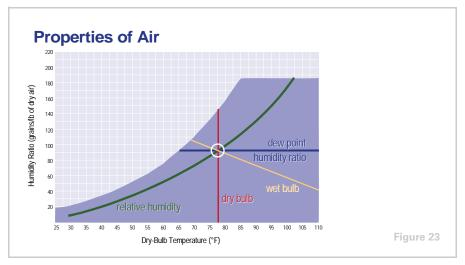
The psychrometric chart now defines these five properties of air: dry-bulb temperature (vertical lines), humidity ratio and dew-point temperature (horizontal lines), relative humidity (curved lines) and wet-bulb temperature (diagonal lines).
