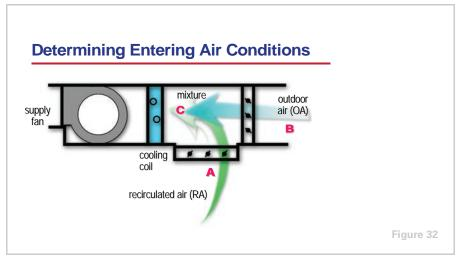
The air entering the cooling coil may be 100% recirculated ( $\bf A$ ), 100% outdoor ( $\bf B$ ), or a mixture of the two ( $\bf C$ ).
