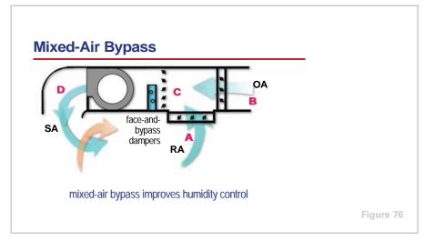
Another method of improving the constant-volume system's ability to control room humidity is to bypass mixed air around the cooling coil. In this example, face-and-bypass dampers are placed in front of the cooling coil and used to vary the portion of the supply air that actually passes through the coil, thus
