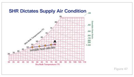
Supply air with any combination of dry-bulb and wet-bulb temperatures that falls on this line will be able to absorb the room's sensible and latent heat in the correct proportions needed to maintain the desired room conditions (**A** = 78°F DB, 65°F WB).
