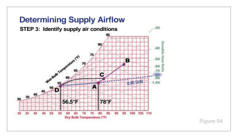
The third step is to determine the required supply air conditions. This is where the coil curves are used. Using the curvature of the nearest coil line as a guide, draw a curve from the mixed-air condition **C** until it intersects the SHR line.
