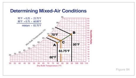
In Period Two, a method was discussed to determine the resulting properties of an air mixture. By plotting the conditions of the **outdoor air** and **recirculated air**, and using the percentage of outdoor air, the resulting condition of the air mixture was calculated and plotted on a straight line from **A** to **B** connecting the two air conditions.
