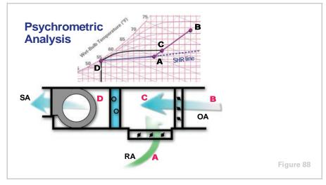
The resulting psychrometric chart plot represents the changes that a volume of air undergoes as it travels through a typical air conditioning system.
