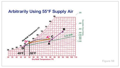
Plotting this new SHR line on the psychrometric chart, we find that the SHR line crosses the coil curve at approximately 49°F DB (**D**).
