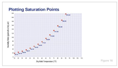
These saturation points can be plotted on a chart with dry-bulb temperature along the horizontal axis and humidity ratio along the vertical axis.
