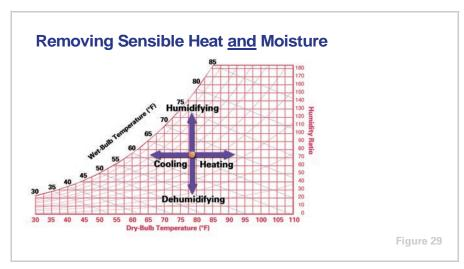
Put all of these changes together on one chart and they show the direction the air condition will move when the dry-bulb temperature or moisture content is altered.
