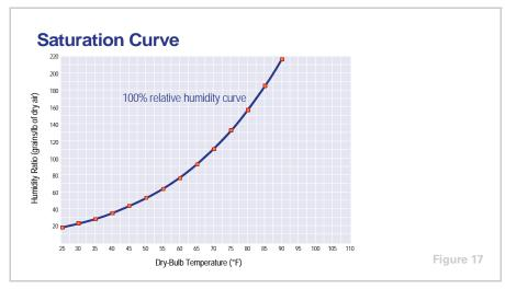
In fact, this curve forms the 100% relative-humidity curve or **saturation curve**. All points on this curve represent the moisture content that constitutes complete saturation of air at the various dry-bulb temperatures.
