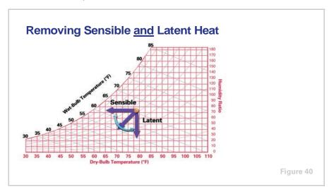
If both sensible and latent heat are removed from the air, the resulting air condition will be to the left and below the initial condition. The proportions of sensible and latent heat removed will determine the exact direction the resulting air condition follows.
