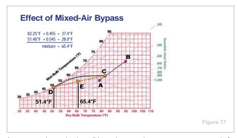
At our example part-load conditions, the room thermostat assumes control of the face-and-bypass dampers, which reduces the amount of air passing through the cooling coil. Since the coil is now "running wild," the reduced airflow through the coil (1,870 cfm) is cooled and dehumidified more than at full load (**D**). When the conditioned air mixes with the bypass air (1,560 cfm), the required supply air condition (3,430 cfm at **E**) results.
