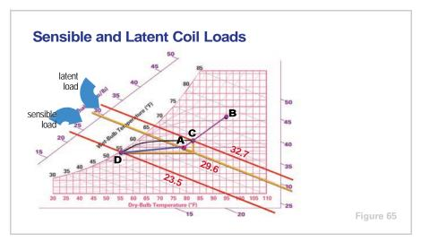
The psychrometric chart can also be used to determine the sensible and latent components of the coil's refrigeration load.
