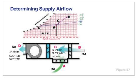
The cooling coil must cool and dehumidify 3,430 cfm of air from the entering condition  $\bf C$  to the supply air condition  $\bf D$  to maintain the desired room conditions.
