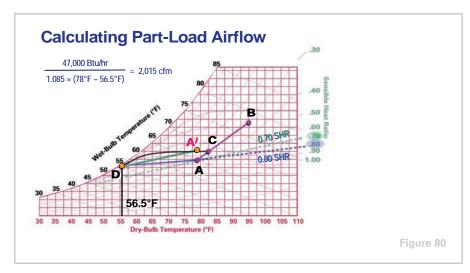
At part load, when the SHR of the room is reduced from 0.80 to 0.70, the VAV system responds by reducing the quantity of 56.5°F air supplied to the room to match the reduced sensible heat gain. The part-load sensible heat gain of 47,000 Btu/hr and the constant supply air temperature, 56.5°F DB, are used to determine the required part-load air quantity.
