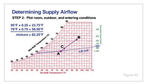
Plot the outdoor air **B** (95°F DB, 78°F WB) and indoor air **A** (78°F DB, 65°F WB) conditions on the psychrometric chart. Then calculate the mixed-air conditions using the method learned in Period 2.
