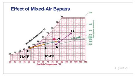
This supply air **E** mixes with room air along the part-load 0.70 SHR line, arriving at the resulting new room conditions **A'**. While the quantity and temperature of supply air are suitable to absorb the room's sensible heat gain, they are unable to completely absorb the latent heat gain. The result is a shift in room conditions from the design point **A** to 78°F DB, 58% RH (**A'**).
