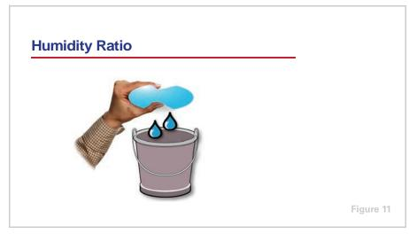
Finally, **humidity ratio** describes the actual weight of water in an air – water vapor mixture. In other words, if one pound of air were wrung completely dry, comparing the weight of the water to the weight of the dry air would yield its humidity ratio.
