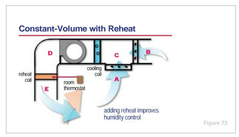
One method of improving the constant-volume system's ability to control room humidity is to reheat the supply air. In this example, reheat is provided by a heating coil located downstream of the air handler. This reheat coil is controlled by a thermostat sensing the room dry-bulb temperature, while the cooling coil is controlled to provide a constant leaving-air temperature.
