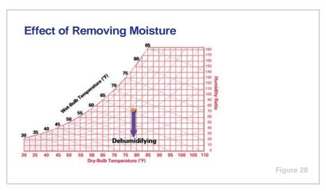
Finally, if moisture is removed from the air without changing its dry-bulb temperature, the air condition moves downward along a dry-bulb temperature line.
