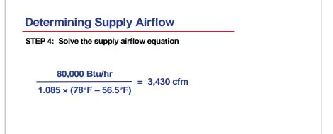
For this example, the supply airflow is calculated as follows:
