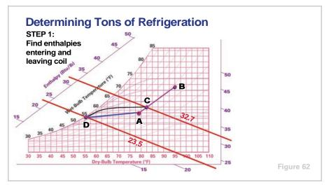
Using the previous example for calculating supply airflow, the first step is to determine the enthalpies of the air entering and leaving the cooling coil. This is accomplished by lining up three points on the chart, including the entering-air condition and identical points on the two enthalpy scales — one each on the left and right edges of the psychrometric chart.
