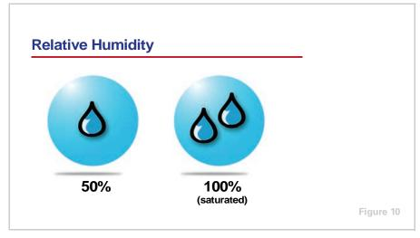
Relative humidity is expressed as a percentage. For example, if the relative humidity of the air is 50%, it contains one-half the amount of moisture possible at the existing dry-bulb temperature.
