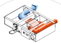
The model FEU is specifically designed for installation in office building corridors, with air inlet and outlet on the same side. Service to the units can be done without disturbing the office occupants.
