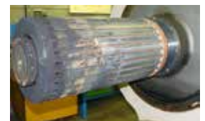
HIGH LEVEL OF OIL ACIDITY Corrosion on the motor windings resulting in motor burn out
