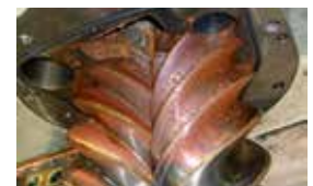
MOISTURE PRESENCE Moisture in oil considerably decreases the lifecycle roller bearings, can lead to corrosion and big damages
