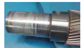
COMPONENTS WEAR High wear on bearing causing compressor failure
