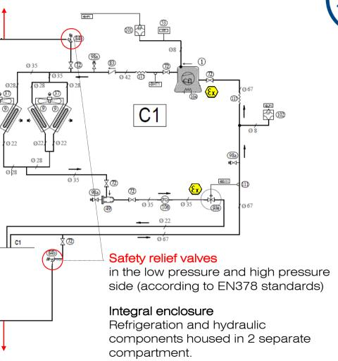
Safety valves discharge outlet (LP)
