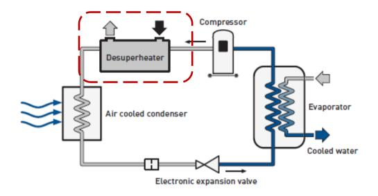
Desuperheater (PHR) = Energy saving by recovering and reusing heat from the refrigeration cycle
