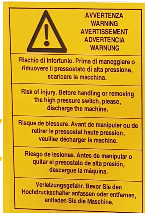
Figure 1 – Indicative position of the signs warning about the necessity of replacing the high pressure switches with the unit void of refrigerant related to the lack of high pressure safety valves
